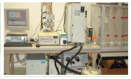
Figure 4: Automated SFC prep system. AutoPrep on Berger Multigram with Knauer UV and ALP.
