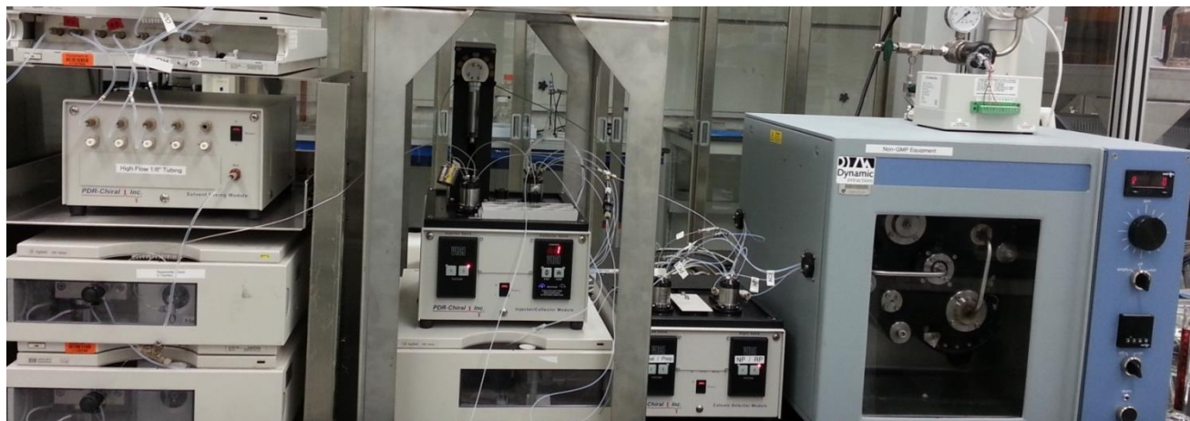
AutoCCC with 2 Agilent 1100 ® analytical Pumps/DAD and Spectrum ® from Dynamic Extractions
