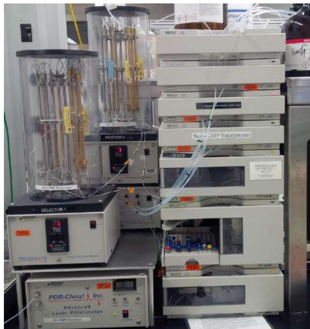
AutoMDS on Agilent with old-style column selectors: 10 bottles/12 columns HILIC on left; and 10 bottles/24 columns Chiral on right with one column selector for neutral and the other for acid additives.
