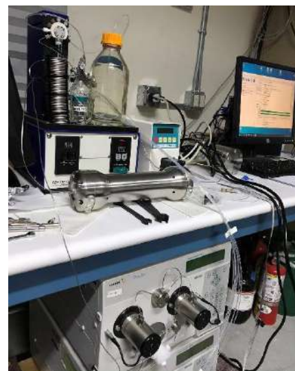
AutoPrep with SD1 pumps and Knauer UV
