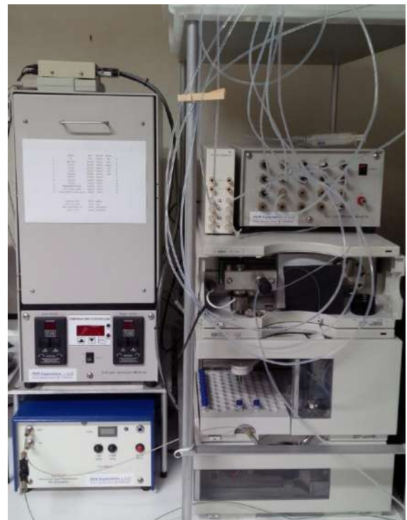
AutoMDS on Agilent with ALP, 20 bottles/24 columns
