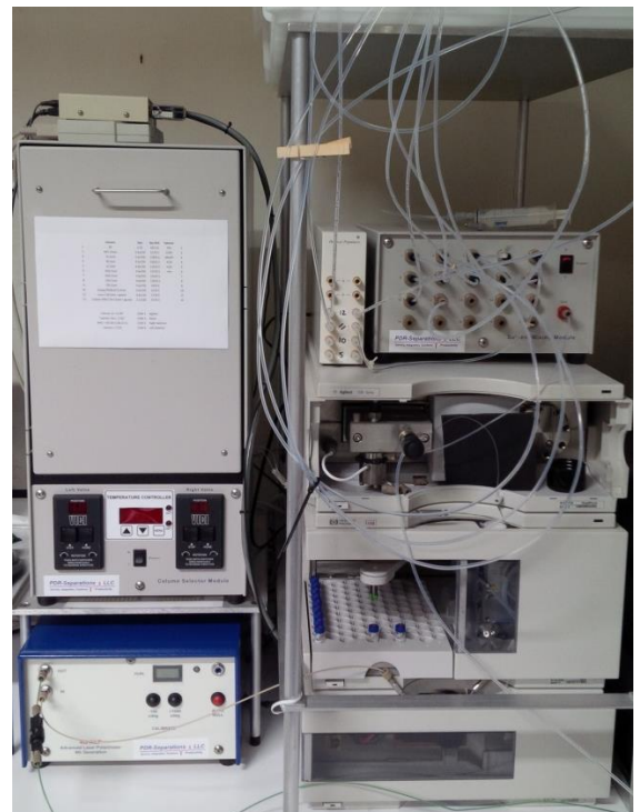
AutoMDS on Agilent with ALP, 20 bottles/24 columns
