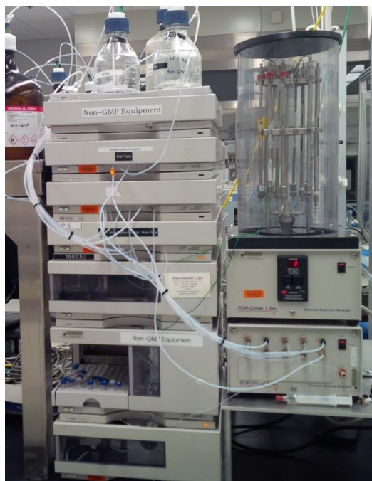
AutoMDS on Agilent with old-style column selectors: 10 bottles/12 columns HILIC on left; and 10 bottles/24 columns Chiral on right with one column selector for neutral and the other for acid additives.
