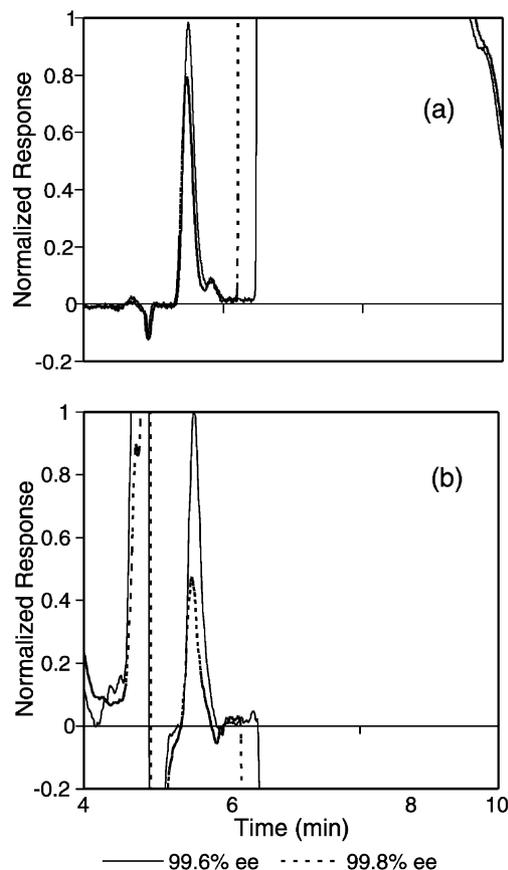
Fig. 5. Comparison of normalized response obtained from 99.6 and 99.8%ee mandelic acid injections using UV/Vis (a) and laser-based polarimetric and (b) detector responses.
