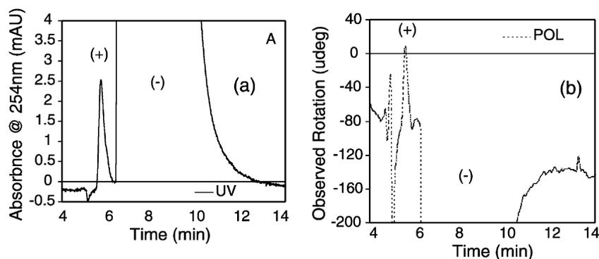
Fig. 4. UV/Vis (a) and laser-based polarimetric (b) detector responses for a chromatographic injection of 20  $\mu\text{l}$  of a 99.80% ee mandelic acid standard. The mandelic acid enantiomers were separated on a Chirobiotic T  $250 \times 4.6$  mm chromatography column at a flow rate of 1.00 ml/min with a mobile phase composition of 1% TEAA pH 4.0.
