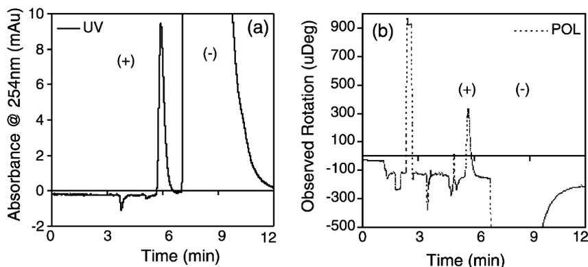
Fig. 3. UV/Vis (a) and laser-based polarimetric (b) detector responses for a chromatographic injection of 20  $\mu\text{l}$  of a 98.00% ee mandelic acid standard. The mandelic acid enantiomers were separated on a Chirobiotic T 250  $\times$  4.6 mm chromatography column at a flow rate of 1.00 ml/min with a mobile phase composition of 1% TEAA pH 4.0.
