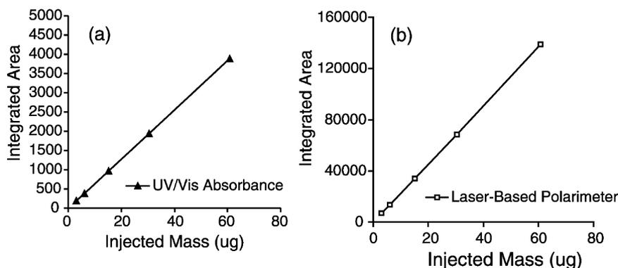
Fig. 2. Linear calibration plots for (R)-(-)-mandelic acid utilizing UV/Vis absorbance detection (a) and laser-based polarimetric detection (b).
